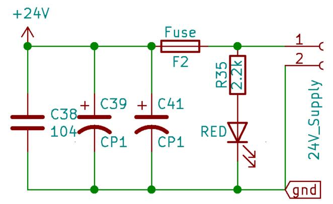
The circuit used for the 24V supply is a simple one which consists of only a fuse protection and some capacitors with an LED indicator. The 24V supply is used by the motor driver L298N, the DC Motors and the battery indicator.
