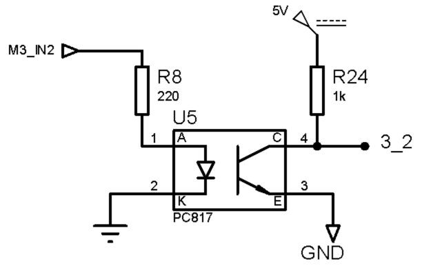
The above shown circuit is for the signal M3\_IN2. When the signal M3\_IN2 is high, the diode AK is activated due to which the CE terminals start conducting and therefore the output signal 3\_2 will be low. Similarly, when the signal M3\_IN2 is low, the diode is in OFF state and the CE terminal acts as an open circuit. Therefore, the signal 3\_2 will be connected to the 5V supply through the 1K resistor.
