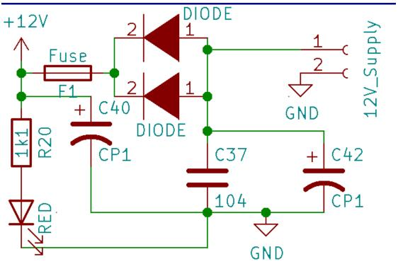
The 12V\_Supply is directly connected to the positive and negative terminals of the 12 V lead acid battery. The two diodes in parallel prevent any reverse current to flow back to the battery. The parallel configuration of diodes allow much higher current to flow through it.
