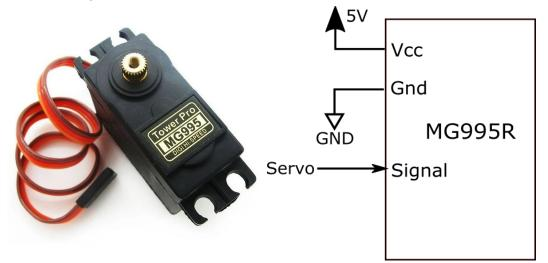
Here, the only signal input to the servo is the Servo signal from the Arduino. The signal is a PWM signal whose duty cycle determines the angle of the servo motor shaft.
