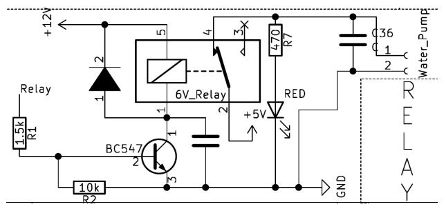
The Relay signal is an input signal from the Arduino. When the Relay signal is high (5v), the transistor turns on which turns on the relay and which in turn turns on the water pump. The signal lines 1 and 2 (in the above fig) are connected directly to the Vcc and Ground wire of the DC water pump. The capacitor C36 is used as a decoupling capacitor for the water pump. The led RED is used as an indicator for when the water pump is ON or OFF.
